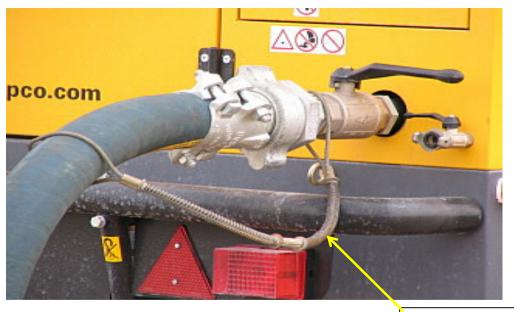
Whip check hose to valve connection
